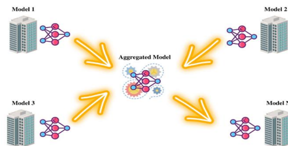
Fig. 1: Use of FL across the organizations. All the models trained by different organizations are aggregated by the server to get the final result (Mammen, 2021)
